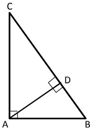
$$\begin{aligned}AD^2 &= BD \times CD \\AB^2 &= BD \times BC \\AC^2 &= CD \times CB\end{aligned}$$
