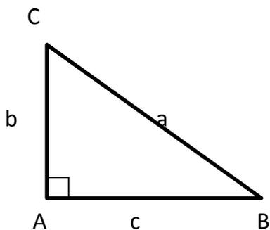
$$\begin{aligned}(BC)^2 &= (AB)^2 + (AC)^2 \\&\text{atau} \\a^2 &= c^2 + b^2\end{aligned}$$
